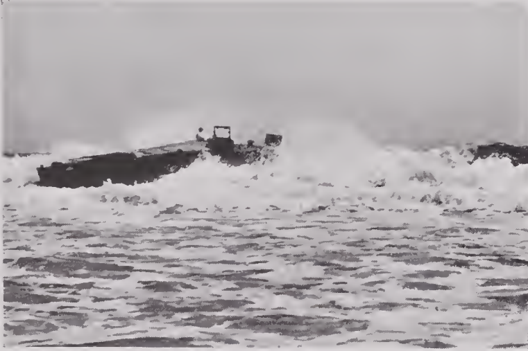
FIGURE 39. First pilot model 2½-ton, 6x6 DUKW in moderate surf.
